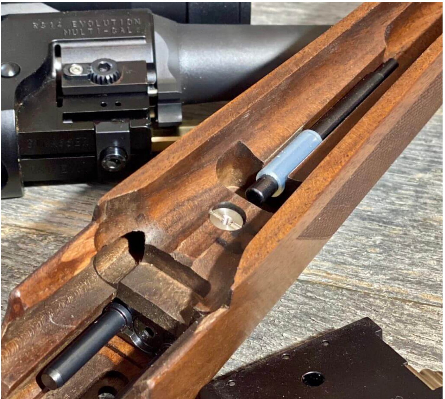
Barrel clamp lever rod is stored in a forearm recess
