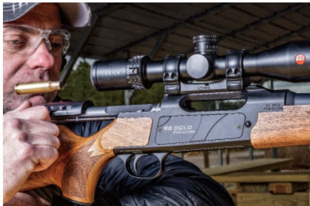
The short, linear movement involved in unlocking the bolt is what makes straight-pull rifles such as the Strasser RS Solo Evolution so fast ($3,451, strasser-usa.com ). Once the handle moves rearwards about 2 inches, the entire bolt assembly moves with it.
