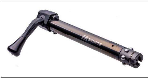
Savage's Impulse features "Hexlock." The removeable bolthead has six stainless-steel ball bearings that act as lugs to lock it into battery.
