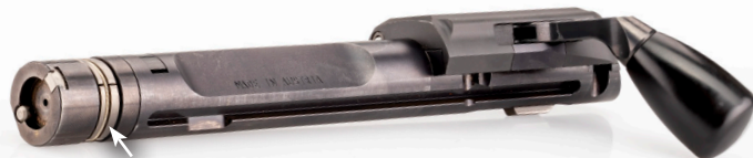
The RS 700's bolt features four lugs (arrow) that lock into place within the barrel. When the bolt is run home and the handle pivoted forward, a sleeve surrounding the firing pin presses the lugs outward to engage mating barrel recesses.
